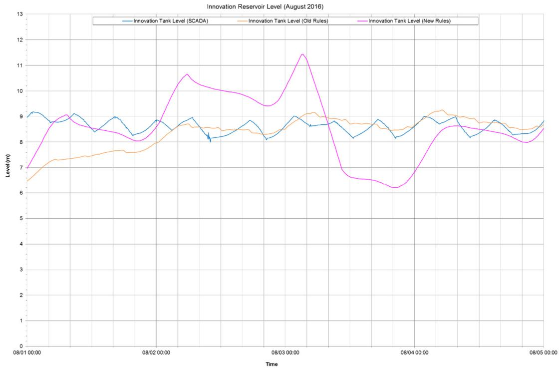
Figure 1-8b SCADA and Model Results on Tank Cycling Profile
